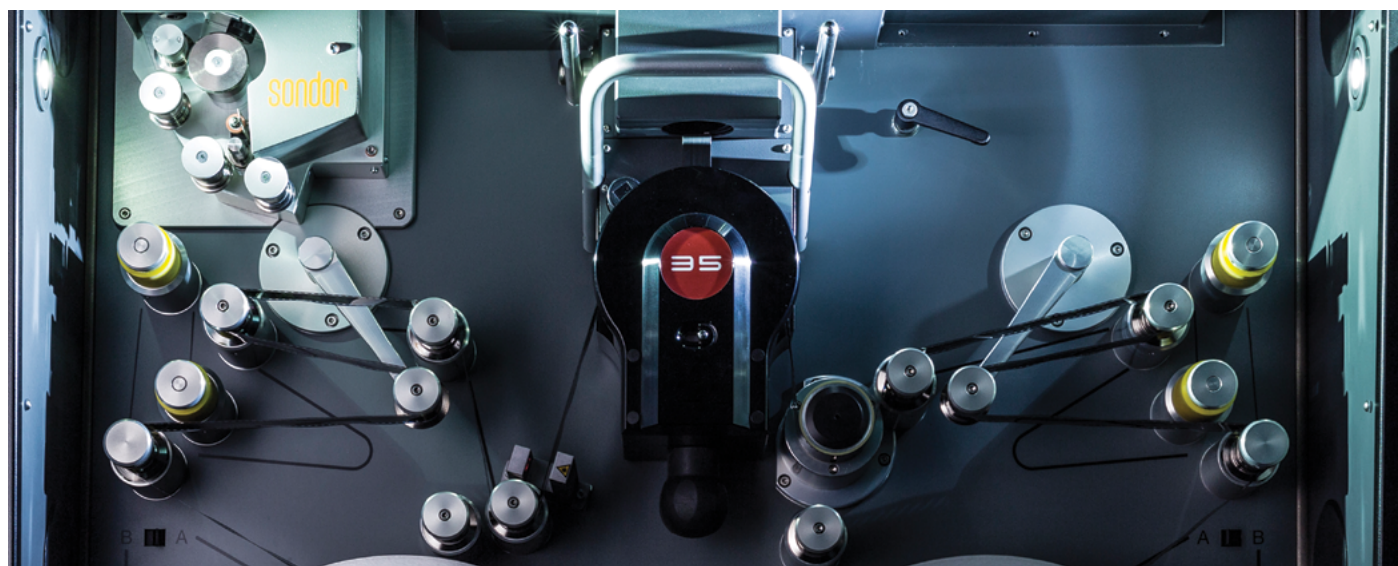
Figure 6 Scanity film transport system
